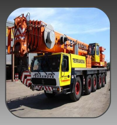
A good all round crane with 51 metres Main boom and all steer capabilities Also comes with additional cwt for heavy lift duties
